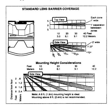
Standard Broad Coverage. Five pair of zones 40' feet wide at widest point and 40' feet out at center. Three pair of sabotage zones in lower field.
