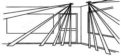
**Testing PIRs.** Walk test all PIRs across the pattern as shown at right to check for activation within the desired patterns.
