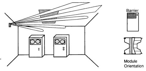
**Permanent Mounting.** Select a mounting height (between 3 and 6 feet) and location which avoids common sources of false alarms, yet maximizes detection potential.
